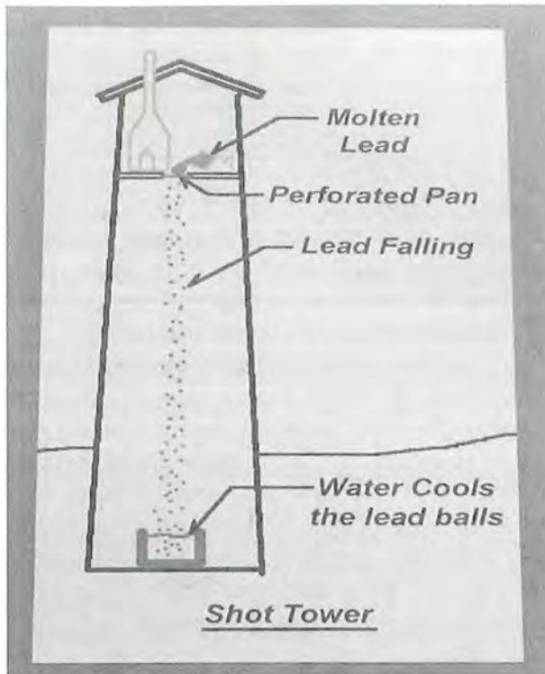
In a shot tower, lead is heated until molten, then dropped through a copper sieve high in the tower. The liquid lead forms tiny spherical balls by surface tension, then solidifies as it falls. The partially cooled balls are caught at the floor of the tower in a water-filled basin. The now fully cooled balls are checked for roundness and sorted by size; those that are "out of round" are
