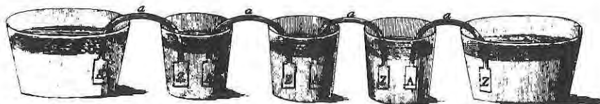
Fig. 26-4. Volta's crown of cups. The "pile" of pairs of zinc and silver discs that formed Volta's first electric battery was modified to form a series of cups filled with weak acid. These were connected by metallic strips terminating in alternate plates of silver (A) and zinc (Z). Reduced evaporation extended the battery's usefulness. (From Transactions of the Royal Society , June, 1800. Courtesy of Burndy Library )
